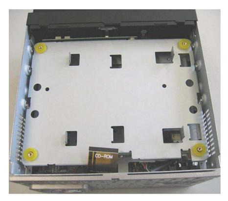
Then the long, golden spacers get removed. The SATA adapter gets screwed of the rear of the mounting unit:
