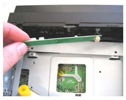
Remove the 2 screws at the sides (red quadrangle in the middle). The 2 other red marked plastic clips have to be pushed in a little, so that you can turn the front forwards:
