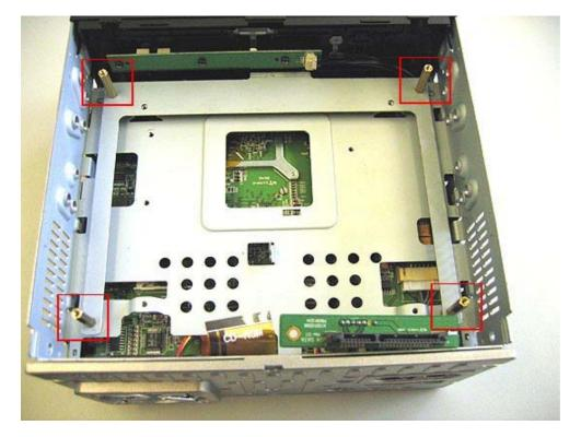
The SATA adapter gets screwed again at the mounting unit and then the HDD gets plugged into its place and gets fastened:
